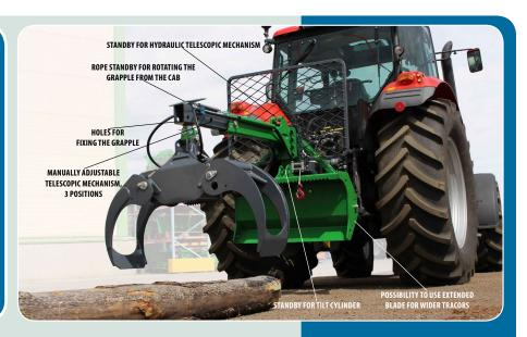
Grapple skidder is available with manual pull-out or hydraulic telescopic mechanism. Operations are possible with the tractor's hydraulics. As an extra option to the grapple skidder, we offer the FARMA winch RW600S that can be controlled via the tractor or via radio control.
